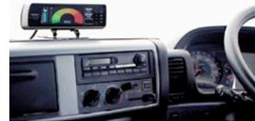
Figure 3. On board weight meter
