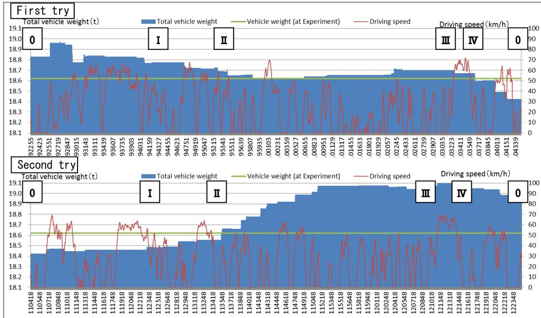
Figure 7. The result of the measurement by the Onboard Mass Unit in anti-clock rotation
