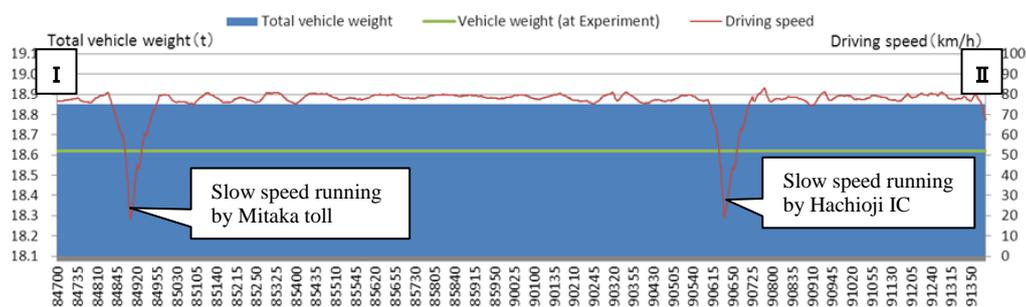
**Figure 10. The result of the measurement by the Onboard Mass Unit in I ~ II Chuo expressway**
