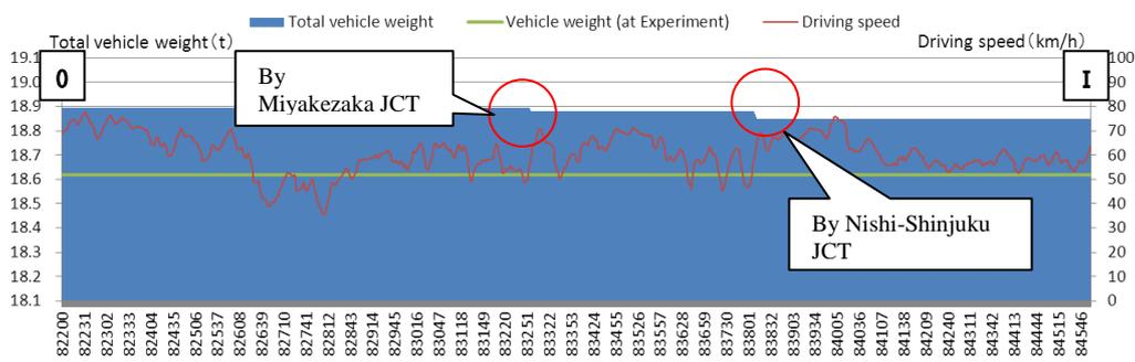
**Figure 9. The result of the measurement by the Onboard Mass Unit in 0~ I Shuto expressway**
