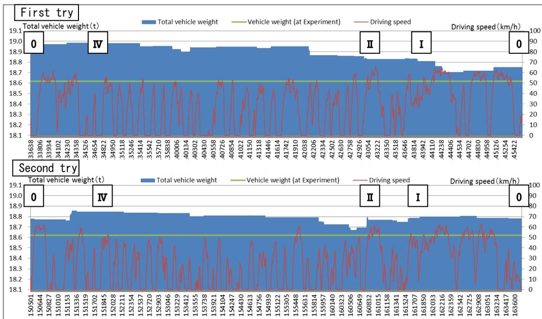
Figure 8. The result of the measurement by the Onboard Mass Unit in clock rotation rotation
