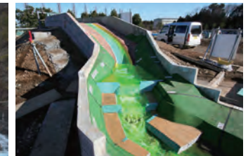
▲ Erosion control experiment with water
